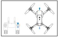
Push the right control stick up and down to fly forward and backwards.
