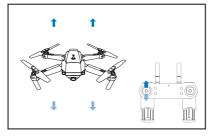
Push the left control stick up to gain altitude and down to descend
