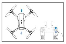
When the drone is hovering in place, and starts to drift forward, press the right control stick backwards until it's stable. If it drifts backwards, press the right control stick forward until it's stable.
