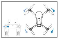
Push the left control stick left and right to pivot left/right.
