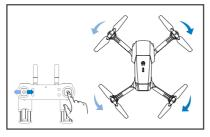
If the drone keeps rotating to left, press the left direction stick to the right until it's stable. If the drone keeps rotating to the right, press the left thumb stick to the left until it's stable.
