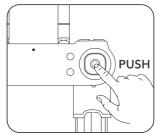
4. To stop trimming, press down on the right control stick again.
